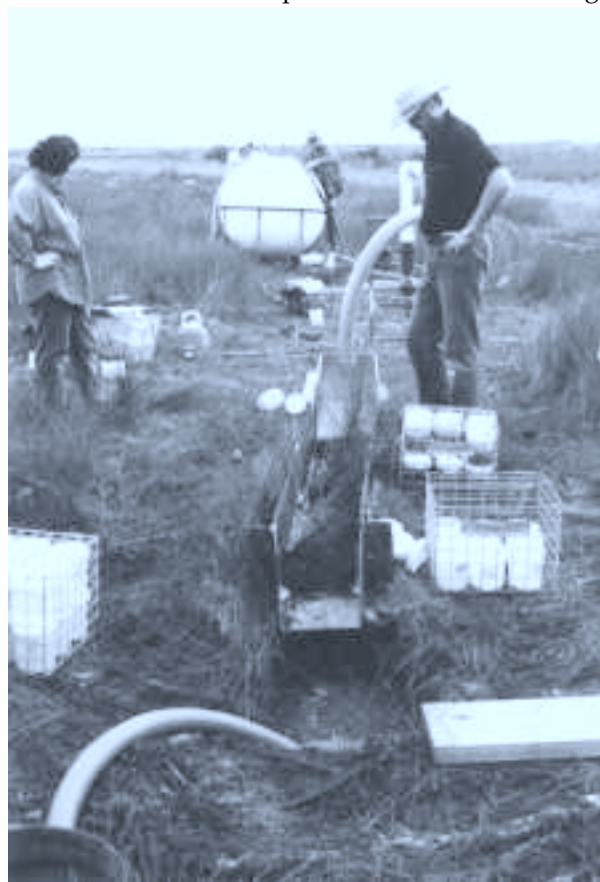
Erosion researchers testing the effectiveness of vegetated filter strips for trapping sediment
